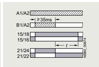
B•¹) 3RP2005-.B OFF-delay with control signal and instantaneous contact
