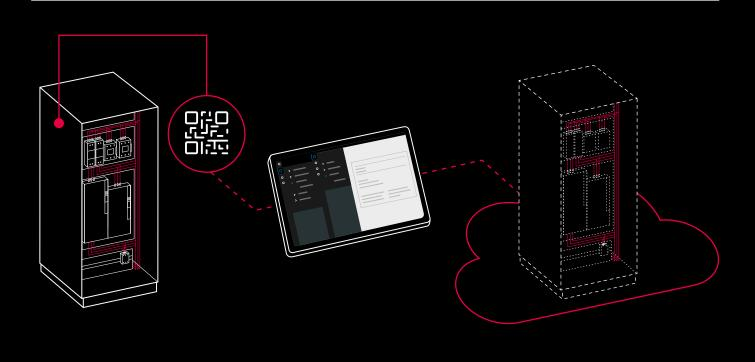
The QR code links physical Rittal enclosures to the digital wiring plan pocket in the EPLAN cloud environment, where all project-specific wiring plan documentation is quickly and conveniently stored.
