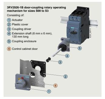
SIRIUS 3RV2926-1B door-coupling rotary operating mechanism
